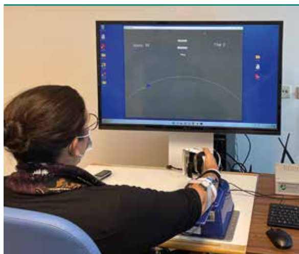
Figure 1. Experimental setup. Participants follow a dynamic target (blue dot on the screen) with and without device support through flexion and extension of the wrist (green dot on the screen)
